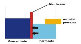
If you reverse this process, by applying more pressure on the higher concentrated solution, clear water flows in reverse direction through the membrane after overcoming the osmotic pressure.
